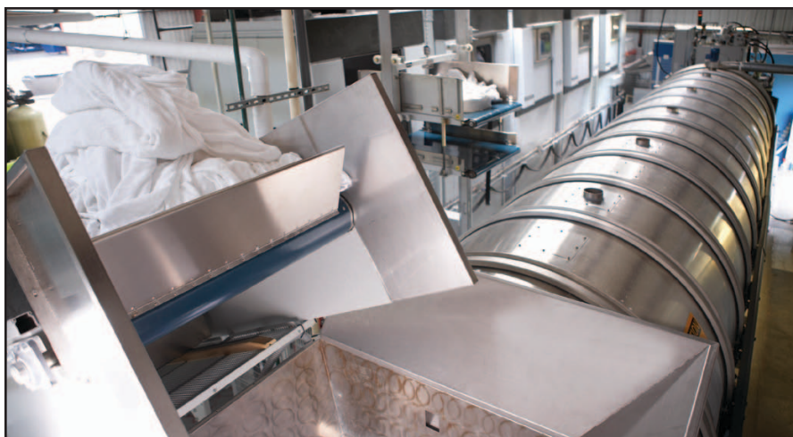
The TBS-50 12-module tunnel washer is top loaded via a conveyor.
